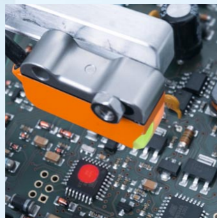
Nothing escapes the photoelectric sensors: Small, slim and flat components, even with dark or shiny surfaces, are detected.
