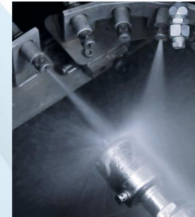
Ingress-resistant under extreme conditions: test for the IP 69K protection rating.
