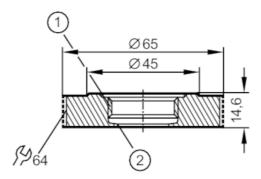
Aseptoflex thread Aseptoflex sealing edge
